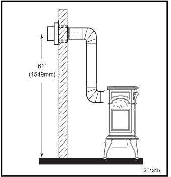
Fig. 21 Minimum wall thimble centerline.
